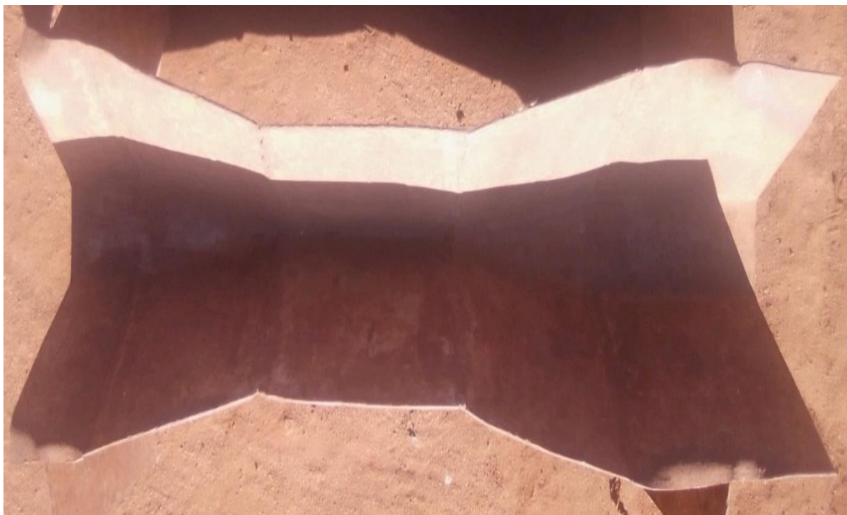
Photo 4.1 Parshall Flume Used to Measure Water Supply into Farmers' Field Plots
